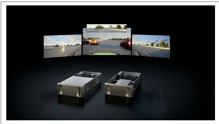
Figure 3-4. The NVIDIA DRIVE Constellation simulation platform uses one server to generate output from sensors, while the other contains the in-vehicle AV computer making driving decisions in real time
